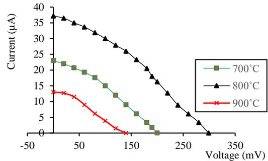
Fig 5. The Illuminated I-V Characteristics of ZnO-Si Heterojunctions at Different Annealing Temperatures
