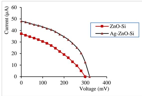
Fig 10. Comparison for the Illuminated I-V Characteristics of ZnO-Si and Ag-ZnO-Si Photo Cells
