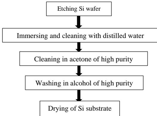
Fig. 1 Block diagram of preparing to growth on Si wafers
