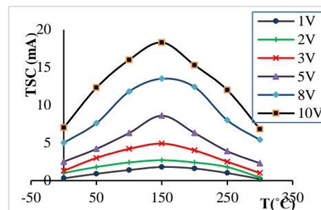
Fig 6. Effect of Biased Voltage on TSC Curves of ZnO-Si Thin Film
