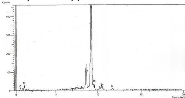
Fig. 2. The Energy Dispersive X-ray (EDX) Analysis of ZnO-Si Sample
