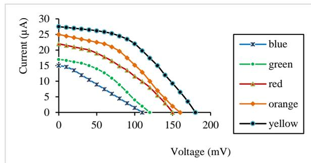
Fig 9. I-V Characteristics of ZnO-Si Cell under Different Wavelengths in Visible Region
