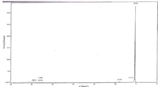
Fig 3. The XRD Pattern of ZnO-Si Sample at Annealing  $800^\circ\text{C}$
