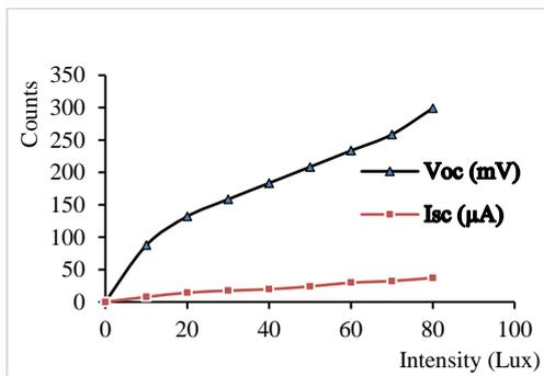
Fig 7. Dependence of  $V_{oc}$  and  $I_{sc}$  on the Illuminated Intensity
